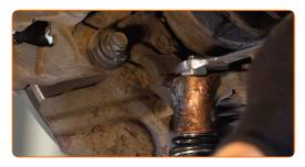
Tighten the arm fastening to the subframe. Use a drive socket #18. Use a combination spanner #18. Use a torque wrench. Tighten it to 100 Nm torque.+90°
