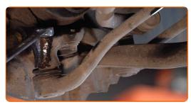
Unscrew the arm fastening from the subframe. Use a drive socket #18. Use a combination spanner #18. Use a ratchet wrench.
