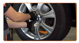
Lower the car and working in a cross order, tighten the wheel bolts. Use a torque wrench. Tighten it to 140 nm torque.
