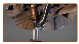
Insert the ball joint into the steering knuckle and fix it with a new nut.
