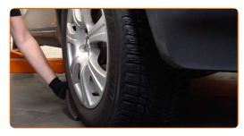
6 Loosen the wheel mounting bolts. Use wheel impact socket #19.
