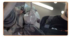
23 Install the brake caliper retaining spring.
