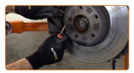
14 Remove the brake caliper.
