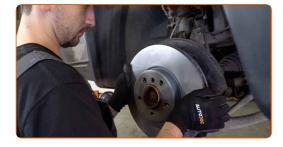
Tighten the brake disc fastening. Use Torx T30. Use a torque wrench. Tighten it to 16 Nm torque.
