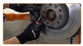
14 Remove the brake caliper.
