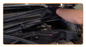
Unscrew the brake fluid reservoir cap.
