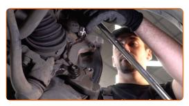
18 Remove the caliper bracket.
