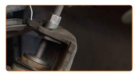
Clean the mounting seats of the caliper and its bracket. Use a wire brush. Use a brake cleaner.
