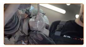
Install the brake caliper retaining spring.
