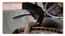
Clean the brake disk surface. Use a wire brush. Use WD-40 spray.
