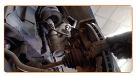
Tighten the brake caliper bracket. Use a drive socket #16. Use a torque wrench. Tighten it to 110 Nm torque.
