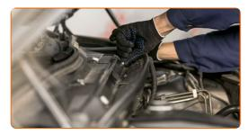
9 Remove the fender protection cover.
