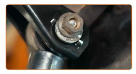
Screw in the fasteners connecting the control arm to the rear knuckle. Use a combination spanner #18. Use a drive socket #18. Use a ratchet wrench.
