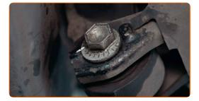
Unscrew the fastener connecting the control arm to the rear knuckle. Use a combination spanner #18. Use a drive socket #18. Use a ratchet wrench.
