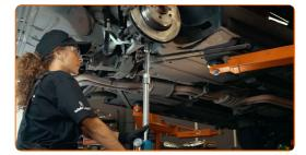
Remove the fastening bolts. Use a pin punch. Use a hammer. Use a crowbar. Use a combination spanner #18.
