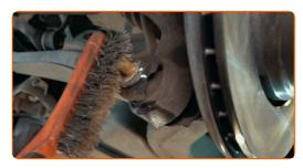
Remove the fastening bolt. Use a drive socket #18. Use a crowbar.
