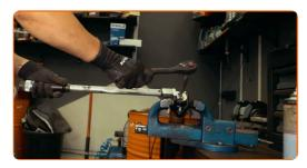
Treat the shock absorber rod fastener. Use copper grease.
