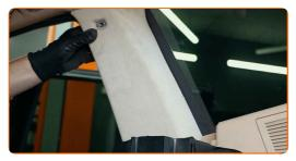
Screw in the fastener of the body pillar trim panel. Use Torx T20. Use a ratchet wrench.
