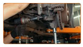
Remove the fastening bolt.
