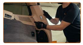
Screw in the fasteners of the plastic car body protective cover. Use a Phillips screwdriver.
