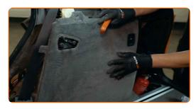
Screw in the fastener of the boot side lining. Use a Phillips screwdriver.
