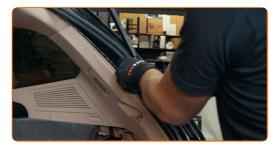
Remove the plastic car body protective cover.
