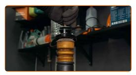
Tighten the shock absorber rod nut. Use a combination spanner #17. Use a shock absorber socket N°DD6. Use an adjustable wrench. Use a torque wrench. Tighten it to 14 Nm torque.
