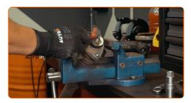
Remove the shock absorber piston rod fastening. Use a shock absorber socket DDNº6. Use a drive socket #16. Use a ratchet wrench.
