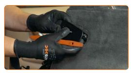
Unscrew the fastener of the boot side lining. Use a Phillips screwdriver.
