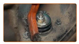
Loosen the upper fastener of the shock absorber. Use a drive socket #13. Use a ratchet wrench.
