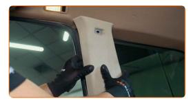
Unscrew the fasteners of the seat belt panel. Use a Phillips screwdriver.
