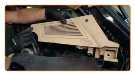
Remove the clips of the boot side lining. Use a plastic trim tool.
