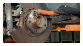
Remove anti-corrosion grease from the new brake disk. Use a brake cleaner.
