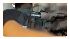
Disconnect the brake pads wear sensor. Use round-nose pliers.
