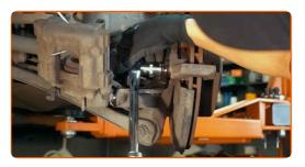
Remove the caliper bracket.
