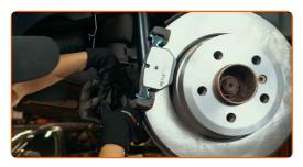
Install the brake caliper and fix it.
