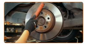
Unscrew the brake disc fastening. Use HEX No.H6. Use an impact screwdriver. Use a rubber mallet.
