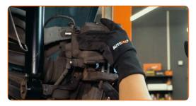
Install the brake caliper retaining spring.
