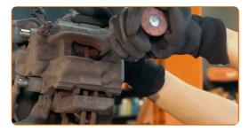
Remove the brake caliper.
