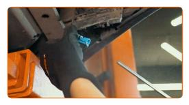
Attach the ABS sensor connector.
