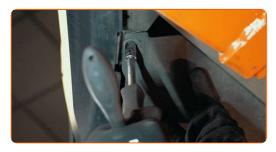
Remove the plastic car body protective cover.
