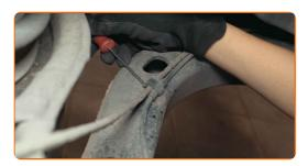
Unscrew the fasteners of the plastic car body protective cover. Use a drive socket #8. Use a ratchet wrench.
