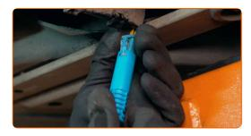
Connect the ABS sensor wiring.
