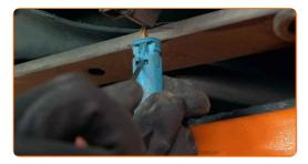
Clean the ABS sensor connector. Use a nylon cleaning brush.
