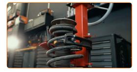
Remove the shock strut mount cap. Use a crowbar.
