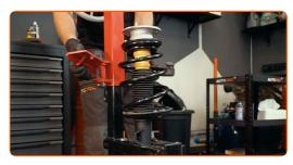
Remove the assembled shock strut.
