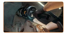
Secure the upper fasteners of the shock strut. Do not tighten it.
