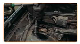
Treat the fasteners of the shock strut mount. Use copper grease.
