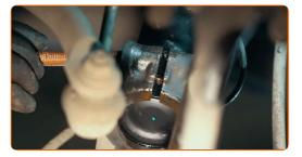
Screw in the fastener that connects the shock strut to the steering knuckle. Use a combination spanner #16. Use a drive socket #18. Use a ratchet wrench.
