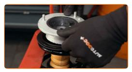
Tighten the shock strut piston rod nut. Use a drive socket #19. Use HEX No.H6. Use a torque wrench. Tighten it to 64 Nm torque.
