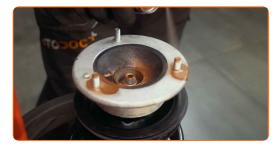
Install the shock strut mount cap.
