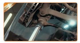
Screw the fastener connecting the control arm to the subframe. Use a combination spanner #16. Use a drive socket #18. Use a ratchet wrench.
