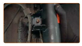
Tighten the fastener connecting the stabilizer link to the shock strut. Use a drive socket #16. Use a torque wrench. Tighten it to 65 Nm torque.
