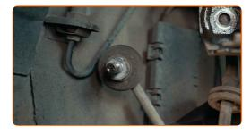
Disconnect the ABS sensor wiring.
