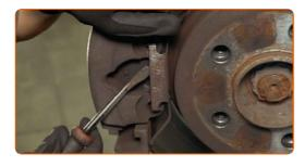
11 Remove the brake caliper.
