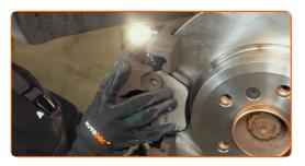
Install the brake caliper retaining spring.
