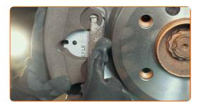
Tighten the brake caliper fasteners. Use HEX No.H7. Use a torque wrench. Tighten it to 30 Nm torque.
