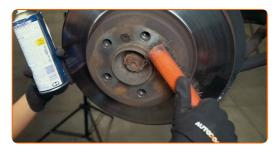
Unscrew the brake disc fastening. Use HEX No.H6. Use an impact screwdriver. Use a rubber mallet.
