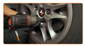
Lower the car and working in a cross order, tighten the wheel bolts. Use wheel impact socket #17. Use a torque wrench. Tighten it to 140 Nm torque.
