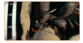
Tighten the fastener that connects the ABS sensor to the steering knuckle. Use HEX No.H5. Use a torque wrench. Tighten it to 7 Nm torque.
