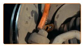
Treat the ABS sensor fastener. Use a multipurpose grease. Use a crowbar.
