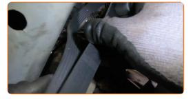
Pull aside the V-ribbed belt tensioner pulley.
