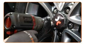
Lower the car and working in a cross order, tighten the wheel bolts. Use wheel impact socket #21. Use a torque wrench. Tighten it to 118 Nm torque.
