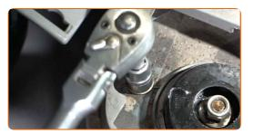
Replacement: suspension strut – Nissan X Trail T30. Tip from AUTODOC:
