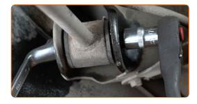
Unscrew the fastener connecting the control arm to the rear knuckle. Use a combination spanner #22. Use a drive socket #22. Use a ratchet wrench.
