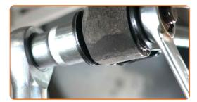
Tighten the fastener connecting the suspension arm to the car body. Use a combination spanner #17. Use a drive socket #17. Use a torque wrench. Tighten it to 98 Nm torque.
