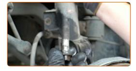
Detach the shock absorber from the rear knuckle. Use a crowbar.
