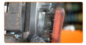
Treat the surface where the brake disc contacts the wheel rim. Use ceramic grease.
