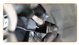
Install the brake hose retaining clip. Use a hammer.
