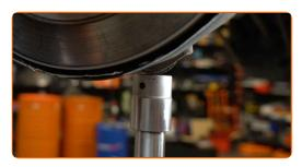
Unscrew the upper fasteners of the shock strut.
