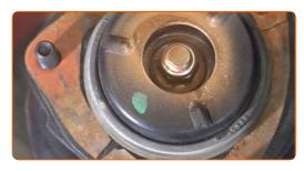
Remove the assembled shock strut.
