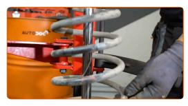
Install the spring on the shock absorber.
