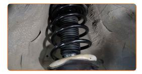
Attach the shock absorber to the rear knuckle.
