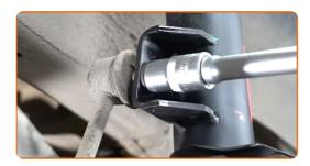
Treat the fastener that connects the sway bar link to the suspension strut. Treat the shock strut fasteners. Use copper grease.
