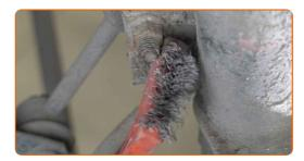
Unscrew the fastener connecting the stabilizer link to the shock strut. Use a drive socket #14. Use a ratchet wrench.
