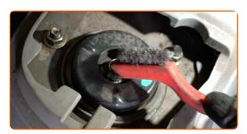
Loosen the suspension strut rod nut. Don't unscrew it completely. Use a drive socket #17. Use a ratchet wrench.
