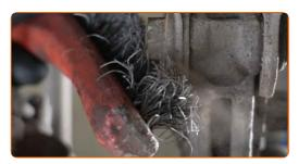
Unscrew the fastener that connects the suspension strut to the rear knuckle. Use a combination spanner #17. Use a drive socket #19. Use a ratchet wrench.
