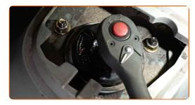
Loosen the upper fasteners of the suspension strut. Use a drive socket #14. Use a ratchet wrench.
