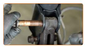
Secure the upper fasteners of the shock strut. Do not tighten it. Use a drive socket #14. Use a ratchet wrench.
