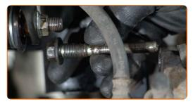
10 Remove the brake caliper.
