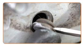
17 Release the parking brake adjuster. Use a flat screwdriver.
