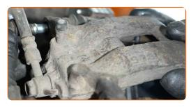
Install the brake caliper guide pins.
