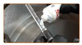
Install the brake caliper and fix it.
