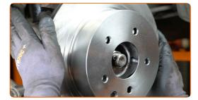
Set the parking brake adjuster in the correct position. Use a flat screwdriver.
