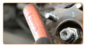
Treat the contacting surface. Use ceramic grease.
