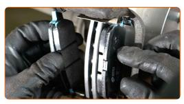
Clean the brake caliper guide pins. Use a brake cleaner.
