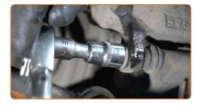
Remove the brake caliper guide pins.
