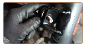
Tighten the fastener connecting the stabilizer link to the stabilizer bar. Use a drive socket #14. Use a torque wrench. Tighten it to 47 Nm torque.
