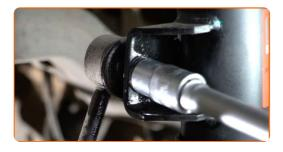
Unscrew the fastener connecting the stabilizer link to the stabilizer bar. Use a combination spanner #15. Use a drive socket #14. Use a ratchet wrench.
