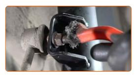
Unscrew the fastener connecting the stabilizer link to the shock strut. Use a drive socket #14. Use a ratchet wrench.
