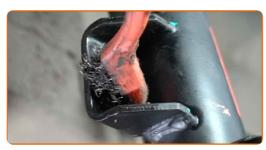
Install a new stabiliser link and tighten the fasteners.
