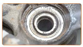
Remove the wheel hub bearing retaining ring. Use a flat screwdriver.
