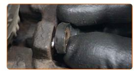
Tighten the fastener that connects the ABS sensor to the steering knuckle. Use a drive socket #10. Use a torque wrench. Tighten it to 9 Nm torque.
