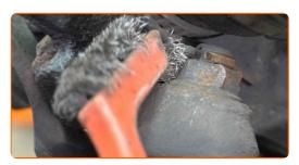
Remove the cotter pin that secures the fastener connecting the ball joint to the steering knuckle. Use a crowbar.
