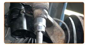
Treat the shock strut fasteners. Treat the fastener connecting the tie rod end to the steering knuckle. Treat the ball joint fastener. Use copper grease.
