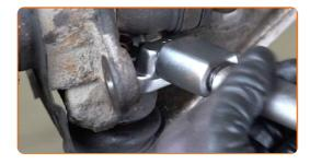
Install the cotter pin that secures the fastener connecting the ball joint to the steering knuckle. Use a crowbar.
