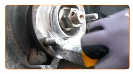
74 Install the brake disc.
