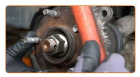
73 Treat the contacting surface. Use ceramic grease.
