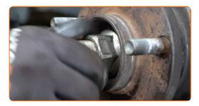
Tighten the fastener connecting the ball joint to the steering knuckle. Use a combination spanner #22. Use a torque wrench. Tighten it to 77 Nm torque.
