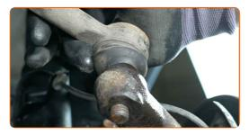
Tighten the fastening nut connecting the tie rod end to the steering knuckle. Use a drive socket #22. Use a torque wrench. Tighten it to 48 Nm torque.
