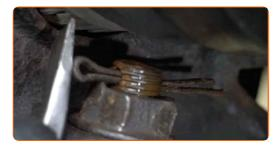
Tighten the lower fasteners connecting the shock strut to the steering knuckle. Use a combination spanner #17. Use a drive socket #19. Use a torque wrench. Tighten it to 140 Nm torque.
