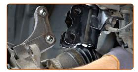
Detach the driveshaft from the steering knuckle.
