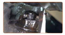
Loosen the fastener connecting the ball joint to the steering knuckle. Use a combination spanner #22.
