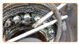
Press out the wheel hub bearing. Bush and bearing driver set.
