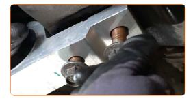
Prop up the steering knuckle. Use a hydraulic transmission jack.
