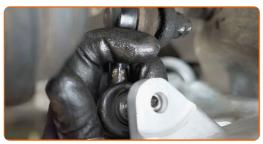
Tighten the fastener connecting the sway bar link to the suspension arm. Use a drive socket #17. Use a torque wrench. Tighten it to 75 Nm torque.
