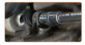
Detach the sway bar link from the suspension arm. Use a crowbar.
