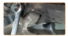
Unscrew the rear fasteners of the arm. Use a drive socket #19. Use a ratchet wrench.
