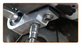
Tighten the front fastener of the arm. Use a combination spanner #22. Use a drive socket #22. Use a torque wrench. Tighten it to 110 Nm torque.
