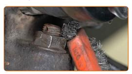
Unscrew the ball joint fastening to the steering knuckle. Use a combination spanner #22.
