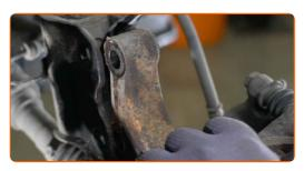
Unscrew the upper fasteners of the shock strut.
