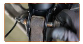
Tighten the lower fasteners connecting the shock strut to the steering knuckle. Use a combination spanner #17. Use a drive socket #19. Use a torque wrench. Tighten it to 140 Nm torque.
