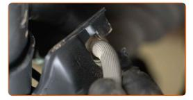
Install the brake hose retaining clip. Use a hammer.
