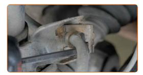
Detach the brake hose from the shock strut.
