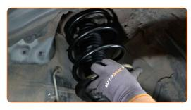
Secure the upper fasteners of the shock strut. Use a combination spanner #14. Do not tighten it.
