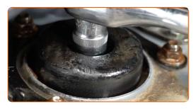
Loosen the upper fasteners of the suspension strut. Use a combination spanner #14.
