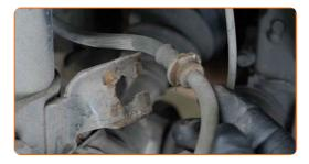
Disconnect the ABS sensor wiring.
