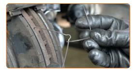
Remove the brake pads. Use a crowbar.
