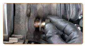
Tighten the brake caliper bracket fasteners. Use a drive socket #22. Use a torque wrench. Tighten it to 148 nm torque.
