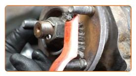
Treat the contacting surface. Use ceramic grease.
