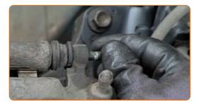
Tighten the brake caliper fasteners. Use a drive socket #14. Use a torque wrench. Tighten it to 32 Nm torque.
