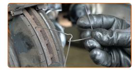
Remove the brake pads. Use a crowbar.
