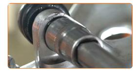
Unscrew the fastener connecting the stabilizer link to the stabilizer bar. Use a combination spanner #17. Use HEX No.H6. Use a ratchet wrench.
