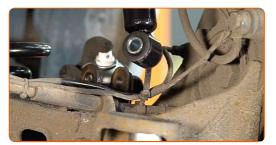
Attach the lower part of the shock absorber. Install the fastening bolt.
