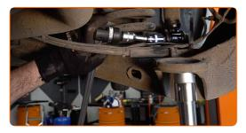
9 Remove the fastening bolt.
