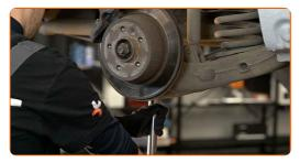
7.1 Clean the shock absorber fasteners.
