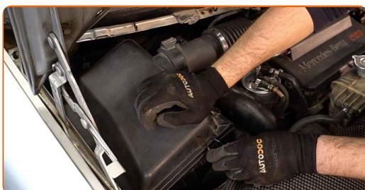
**62** Screw in the fastening screws of the air filter cover. Use a Phillips screwdriver.
