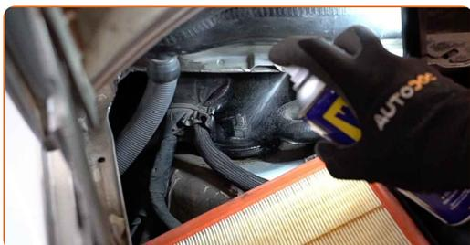
**12** Loosen the upper fastener of the shock strut mount. Use a combination spanner #21. Use HEX No.H6.
