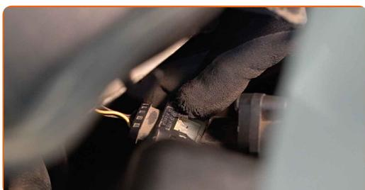
**64** Screw in the fasteners of the vacuum pressure converter valve.
