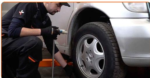
**14** Loosen the wheel mounting bolts. Use wheel impact socket #17.
