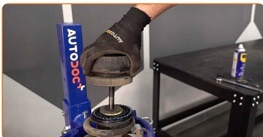
34 Release the coil spring.
