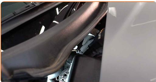
**7** Detach the air intake hose clamp. Use a drive socket #7. Use a ratchet wrench.
