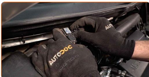
**65** Fasten the clamp on the air intake hose. Use a drive socket #7. Use a ratchet wrench.
