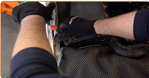
**4** Release the air filter cover clips.
