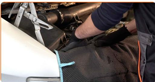
**3** Undo the fastening screws of the air filter cover. Use a Phillips screwdriver.
