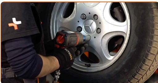
**56** Lower the car and working in a cross order, tighten the wheel bolts. Use a torque wrench. Tighten it to 175 Nm torque.
