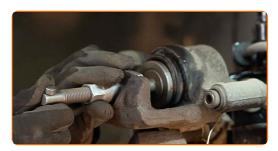
Treat the brake caliper bracket where it contacts the brake pads. Use anti-squeal paste.
