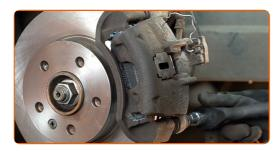
Connect the brake pad wear sensor plug.
