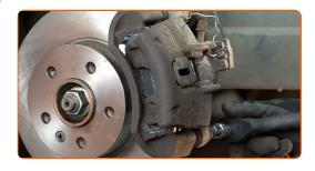
Connect the brake pad wear sensor plug.
