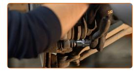
10 Remove the brake caliper.
