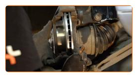
Tighten the brake caliper bracket. Use a drive socket #21. Use a torque wrench. Tighten it to 162 Nm torque.
