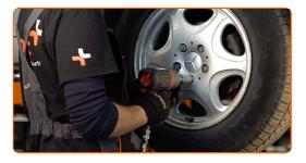
Lower the car and working in a cross order, tighten the wheel bolts. Use a torque wrench. Tighten it to 175 Nm torque.
