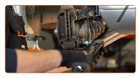
15 Remove the caliper bracket.
