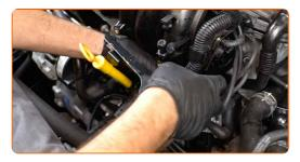
Tighten the fastener of the secondary air pump bracket. Use HEX No.H6. Use a drive socket #13. Use a torque wrench. Tighten it to 9 Nm torque.
