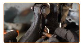
Screw in the fasteners connecting the suspension strut to the steering knuckle. Use a combination spanner #18. Use a drive socket #18. Use a tap wrench.
