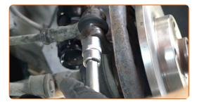
Tighten the lower fasteners connecting the shock strut to the steering knuckle. Use a combination spanner #18. Use a drive socket #18. Use a torque wrench. Tighten it to 95 Nm torque.
