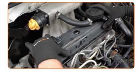
Tighten the engine valve cover fasteners. Use a drive socket #10. Use a torque wrench. Observe the recommended tightening torque.
