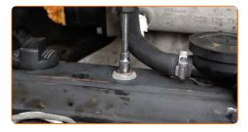
Remove the microfibre cloth from the PCV valve hole.
