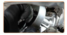
Tighten the water pump pulley fastener. Use HEX No.H6. Use a torque wrench. Observe the recommended tightening torque.
