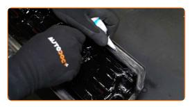
Install the engine valve cover gasket.
