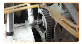
Remove the timing belt tensioner pulley.
