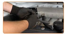
9 Remove the air distribution housing assembly.
