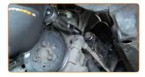
Remove the hydraulic power steering pump.
