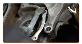
Treat the water pump mounting seat. Use a sealant.
