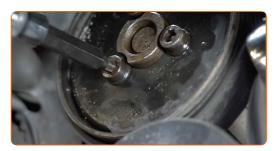
Remove the water pump pulley.
