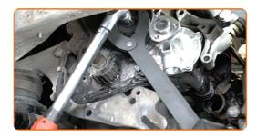
72 Attach the lower coolant pipe.
