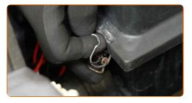
Screw in the fasteners of the air distribution housing assembly. Use a drive socket #7. Use a ratchet wrench.
