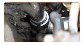
Attach the clip of the lower coolant hose.
