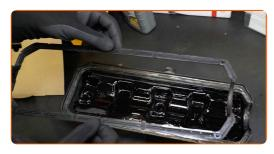
Install the engine valve cover.
