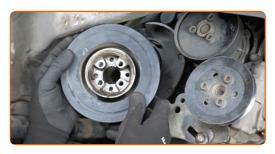
Clean the water pump pulley fastener. Use a wire brush. Use all-purpose cleaning spray.
