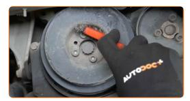
Unscrew the fastener of the crankshaft pulleys. Use HEX No.H6. Use a ratchet wrench.
