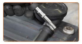
Remove the crankcase ventilation hose.
