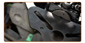
Remove the camshaft locking tool.
