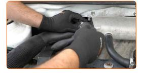
115 Remove the coolant reservoir cap.
