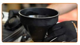
Pour coolant in the coolant reservoir.
