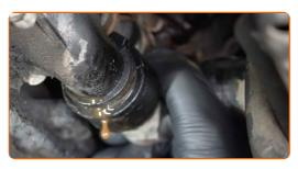
Drain the coolant from the engine.
