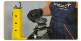
Tighten the shock strut piston rod nut. Use a drive socket #21. Use a torque wrench. Tighten it to 65 Nm torque.
