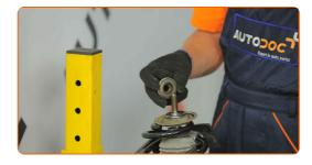
Screw in the fastener of the shock strut mount.
