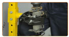
Unscrew the fastener of the shock strut mount.
