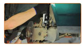
Install the bracket onto the shock absorber strut.
