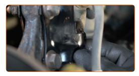
Tighten the brake hose fastening bracket to the shock strut. Use a drive socket #10. Use a ratchet wrench.
