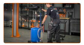
Unscrew the drain plug. Use a drive socket No.19 or ring spanner No.19. Drain the used oil.
