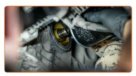
Clean the area of the oil pan drainage hole.
