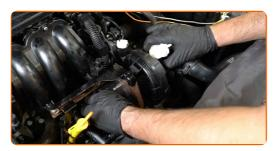
Screw in the fasteners connecting the secondary air pump to its bracket. Use a combination spanner #10.
