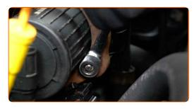
Attach the secondary air pump connector.
