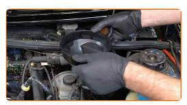
Pour coolant in the coolant reservoir.
