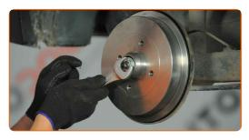
10 Remove the brake drum.
