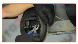
Pull both brake shoes with the adjuster from the working brake cylinder, avoiding damage to the boots.
