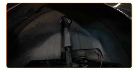
Install the shock absorber mount using the center hole as a guide.
