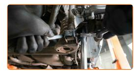
Unscrew the upper fastener of the shock absorber. Use a drive socket #16.
