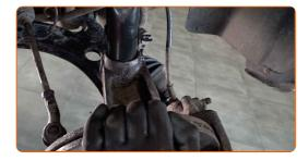
Replacement: strut mount – VW up! Hatchback (121, 122, BL1, BL2). Tip from AUTODOC:
