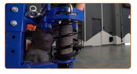
Remove the assembled shock strut.
