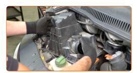
9 Remove the filter element from the filter housing.
