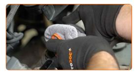
Release the air filter cover clips.
