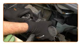
6 Cover the air intake hose with a microfibre towel to prevent dust and dirt from getting into the system.
