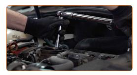
Replacement: spark plugs – VW Transporter VI Platform / Chassis (SFD, SFE, SFL, SFZ). AUTODOC recommends:
