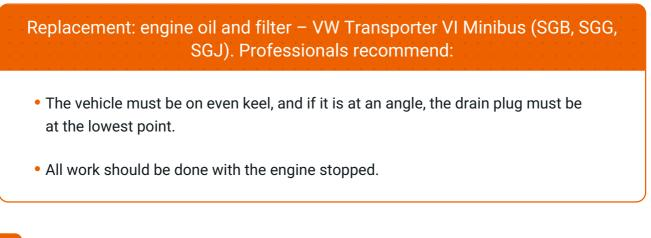
Put a waste oil container with at least 5 l capacity under the drainage hole.
