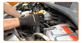
Replacement: fuel filter – VW Transporter VI Minibus (SGB, SGG, SGJ). AUTODOC recommends:
