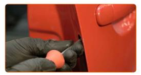
Install the cover on the exterior door handle fastener.
