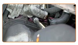
Remove the thermostat housing.
