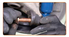
Tighten the lower fastener of the shock absorber. Use a combination spanner #21. Use a drive socket #21. Use a torque wrench. Tighten it to 120 Nm torque.+90°
