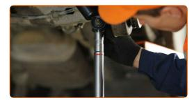
9 Remove the fastening bolt.
