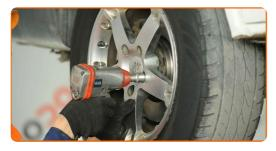
Lower the car and working in a cross order, tighten the wheel bolts. Use wheel impact socket #19. Use a torque wrench. Tighten it to 180 Nm torque.
