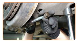
Remove the support from under the arm.
