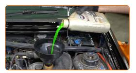
Replacement: engine thermostat – VW Transporter V Platform / Chassis (7JD, 7JE, 7JL, 7JY, 7JZ, 7FD). Tip from AUTODOC:
