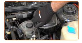
Remove the fender protection cover.
