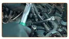
Replacement: glow plugs – VW Transporter V Minibus (7HB, 7HJ, 7EB, 7EJ, 7EF, 7EG, 7HF, 7EC). Tip from AUTODOC experts:
