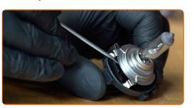
Replacement: headlight bulb – VW Transporter T6 Platform / Chassis (SFD, SFE, SFL, SFZ). AUTODOC recommends:
