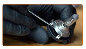
Replacement: headlight bulb – VW Transporter T6 Minibus (SGB, SGG, SGJ). AUTODOC recommends:
