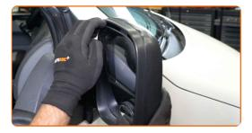
Carefully release the mirror glass from its attachment. Use a plastic trim tool. Use a flat screwdriver.
