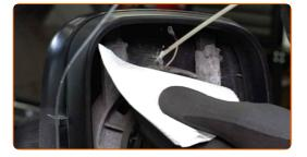
Attach the mirror heating connectors.
